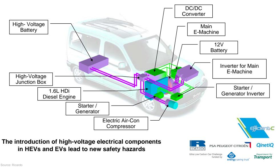
Safety considerations for HEVs and EVs revolve around identifying the hazards from the battery pack, high voltage and quiet operation
